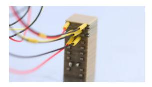
The Noliac shear stack NAC3404-H12.6 features motion in the X/Y/Z-axis. This product is ideal for stick-slip and nanopositioning applications. NAC3404-H12.6 measures 15x15 mm with a height of 12.6 mm and provides free stroke of 3/3/3 µm and a capacitance of 14.9/14.9/92.8 nF. End plates on top and bottom are included. The shear stack has ultra thin electrodes made of standard steel as standard.
