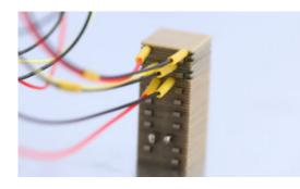
The Noliac shear stack NAC3404-H23.1 features motion in the X/Y/Z-axis. This product is ideal for stick-slip and nanopositioning applications. NAC3404-H23.1 measures 15x15 mm with a height of 23.1 mm and provides free stroke of 6/6/6  $\mu$ m and a capacitance of 29.8/29.8/185.7 nF. End plates on top and bottom are included. The shear stack has ultra thin electrodes made of standard steel as standard.
