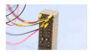
The Noliac shear stack NAC3404-H33.6 features motion in the X/Y/Z-axis. This product is ideal for stick-slip and nanopositioning applications. NAC3404-H33.6 measures  $15 \times 15$  mm with a height of 33.6 mm and provides free stroke of 9/9/9  $\mu$ m and a capacitance of 44.8/44.8/278.5 nF. End plates on top and bottom are included. The shear stack has ultra thin electrodes made of standard steel as standard.
