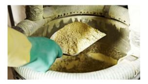
Noliac piezoceramic material NCE41 is a hard doped material with low dielectric and mechanical loss. Combined with a high piezoelectric charge constant (d33), it is suitable for high-performance ultrasonic applications.
