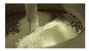
Noliac piezoceramic material NCE46 is a hard doped material, which can be exposed to high electrical and mechanical stresses.
