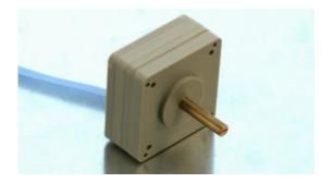
PAD7344 is a low-power motor designed for non-magnetic applications. PAD is a drive technology transforming the linear motion of high performance piezo multilayer actuators into a powerful and precisely controllable rotation. PAD7344 includes four multilayer piezo benders in a non-magnetic structure, providing high performance in a compact package.
